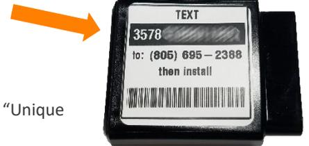
**Step 2:** Plug the tracker into the vehicle’s OBDII port. This will be low down, underneath the dashboard, on the driver’s side. **You should see flashing lights on the tracker** if it is receiving power. If you do not, please check the OBD port’s fuse.
