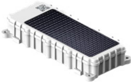
The TLP2-SFB device features an expanded battery capacity and a larger solar panel for improved battery life and more efficient solar recharging. This device is ideal for tracking and monitoring assets such as containers, trailers, trucks, etc.
